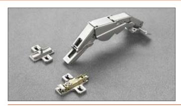
For thicker doors max. 35 mm. Hinge with greater opening angle and reduced operating profile. 11 mm deep die-cast cup. 155° opening.
