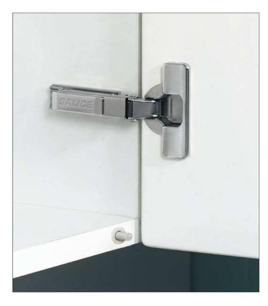
Drill a hole Ø 10 mm and min. 50 mm depth in the cabinet. Insert Smove into the hole.
