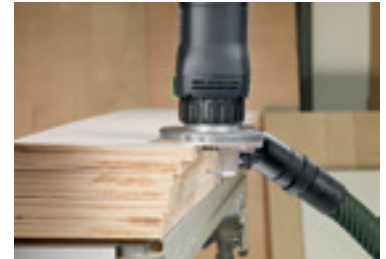
Chamfering plastic or solid wood veneer.
